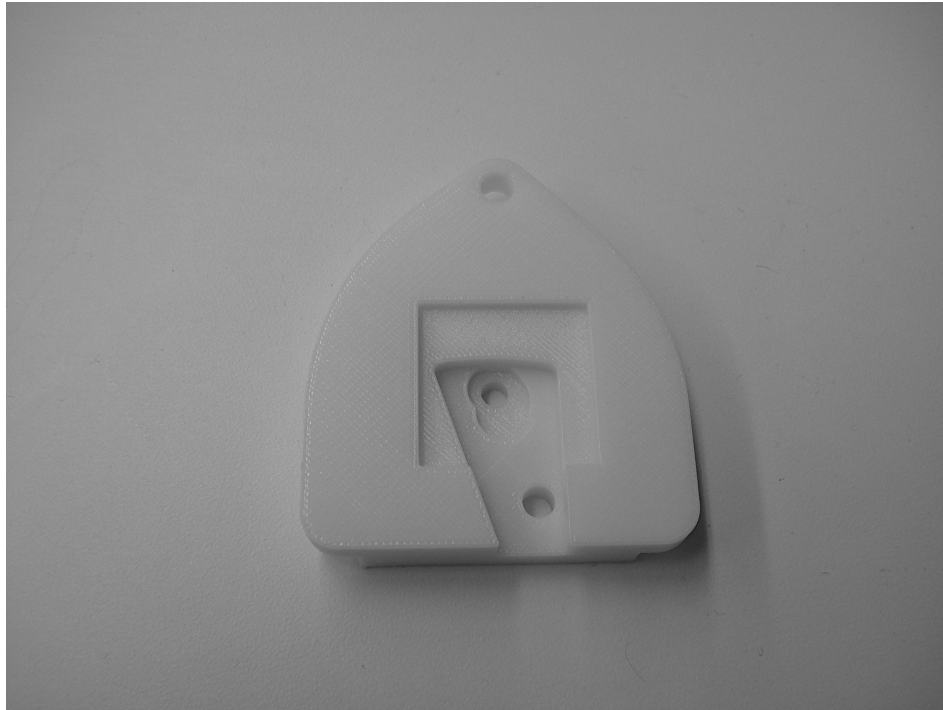
Figure 4.5.1-5 – A part created using the FDM approach to 3D printing (courtesy of Prescient Surgical).
